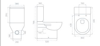
Easy Access Exposed Water inlet (left or right) 4.5/3L Flush Volume Soft Close & Quick Release Seat
