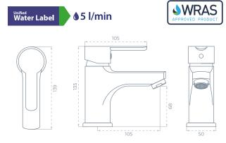
\*\*Pre-fitted 5 I/min flow restrictor requiring a minimum operating pressure of 1 bar Optional low pressure aerator requiring minimum operating pressure of 0.2 bar supplied
